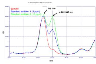
With resolution better than 5 pm even the most challenging spectral interferences can be separated
