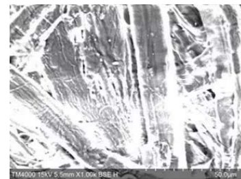
Charging phenomenon occurred during observation!
