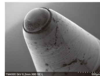
TM4000PlusIII Accelerating voltage: 5 kV Image signal: SE Magnification: 60x Sample: Tip of ballpoint pen
